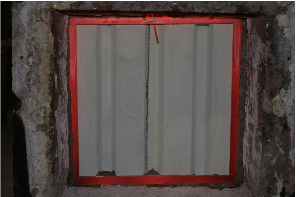
Figure 3.1: Exposed side of specimen after removal from furnace
