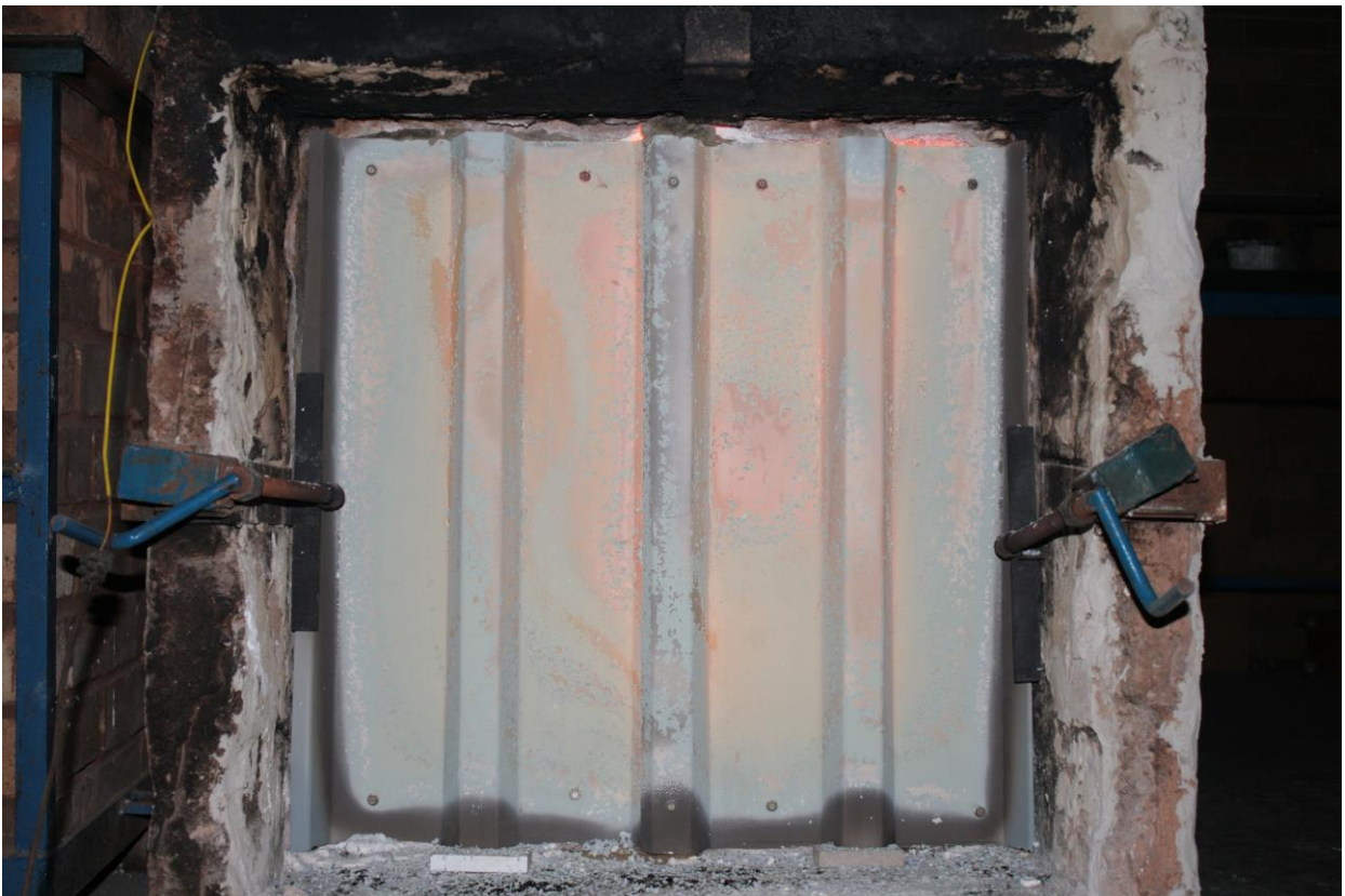
Figure 3.2: Condition of specimen from the unexposed side after conclusion of test
